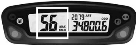
Fig 2 MAX speed function
