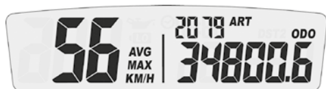
Screen 3: Alternating AVG/MAX speed, Accumulated run time, ODO
