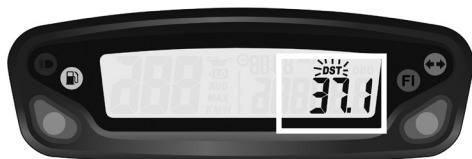
Fig 6 Adjustable trip distance function
