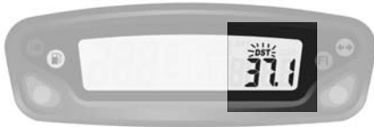
Fig 6 Adjustable trip distance function
