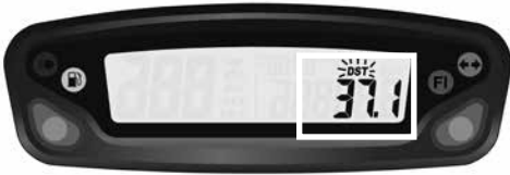
Fig 6 Adjustable trip distance function
