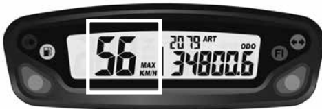
Fig 2 MAX speed function
